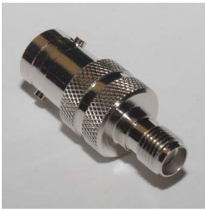
Female BNC to Female SMA (Chinese Radios, Baofeng etc.)
